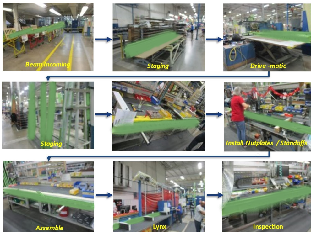
Figure 6: Original floor beam production line using batch processing and parallel build positions.
