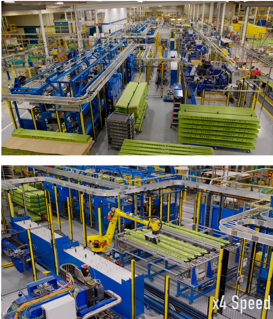
Figure 13: The ABL includes a mix of manual/semi-automated and automated workstations in a takt-based hybrid single-piece flow arrangement.
