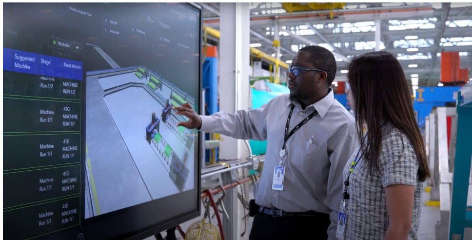
Figure 2: IIoT feeds a digital twin of factory operations enabling constraint-based scheduling.
